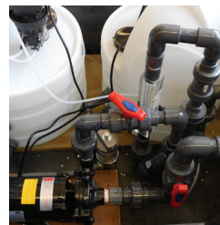
Tanks and injection pump used to apply products at Farmers Grain Terminal
