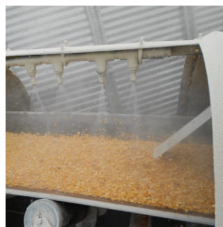
Applying Diacon® IGR and Centynal™ Insecticide directly to the corn grain stream
